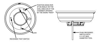
Figure 4. Recessed Test Switch Opening and SENS-RDR Position
